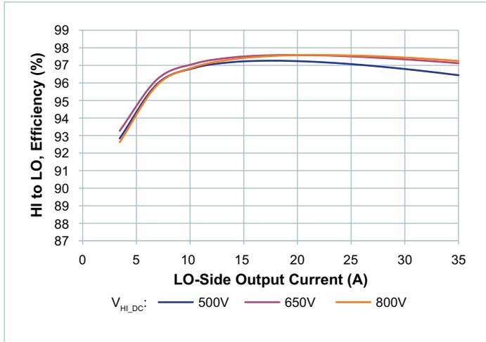
Figure 10 — Efficiency at  $T_{CASE} = 70^{\circ}C$
