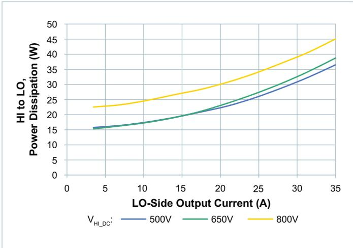
Figure 7 — Power dissipation at  $T_{CASE} = -55^{\circ}C$
