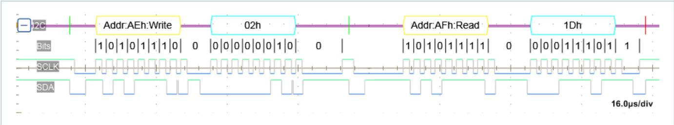
Figure 2 — ON\_OFF\_CONFIG COMMAND (02h), READ BYTE PROTOCOL
