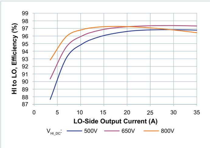
Figure 6 — Efficiency at  $T_{CASE} = -55^{\circ}C$
