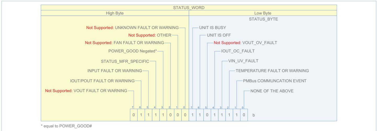
All fault or warning flags, if set, will remain asserted until cleared by the host or once the BCM and VDDDB power is removed. This includes undervoltage fault, overvoltage fault, overvoltage warning, overcurrent warning, overtemperature fault, overtemperature warning, undertemperature fault, reverse operation, communication faults and analog controller shut-down fault.
