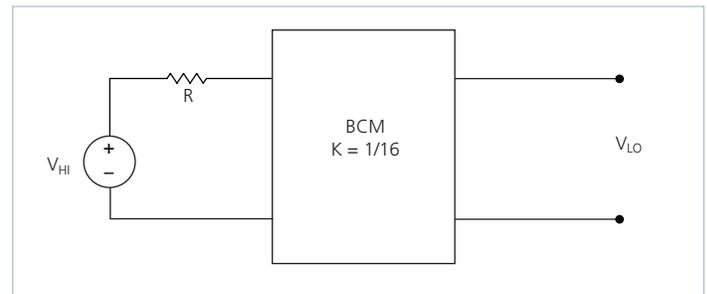
Figure 20 — K = 1/16 BCM with series HI-side resistor
