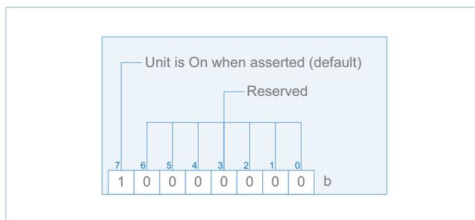
This command accepts only two data values: 00h and 80h. If any other value is sent the command will be rejected and a CML Data error will result.
