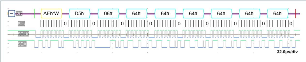
Figure 5 — SET\_ALL\_THRESHOLDS COMMAND (D5h)\_WRITE BLOCK PROTOCOL
