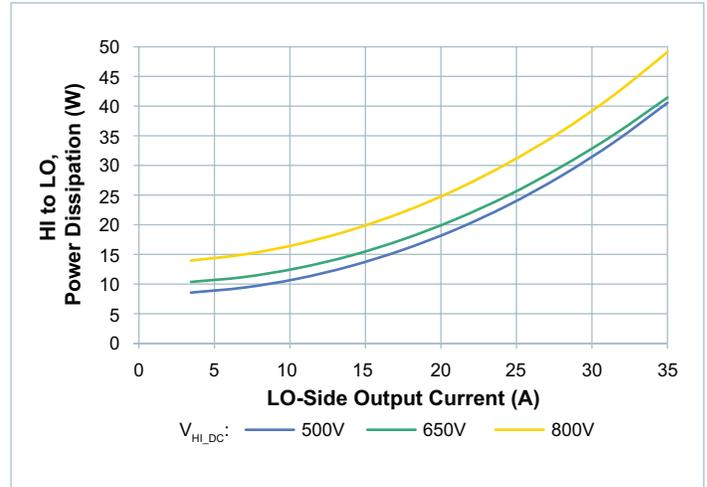
Figure 11 — Power dissipation at  $T_{CASE} = 70^{\circ}C$
