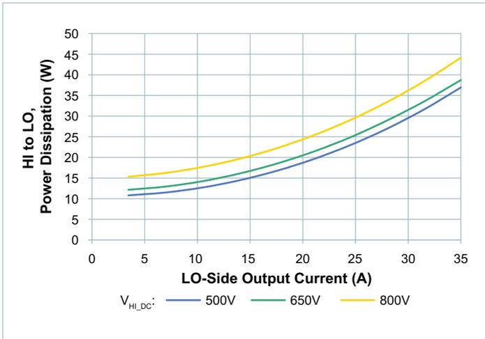
Figure 9 — Power dissipation at  $T_{CASE} = 25^{\circ}C$
