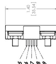
BCM in VIA Package PCB (Board) Mount Package Recommended Hole Pattern
