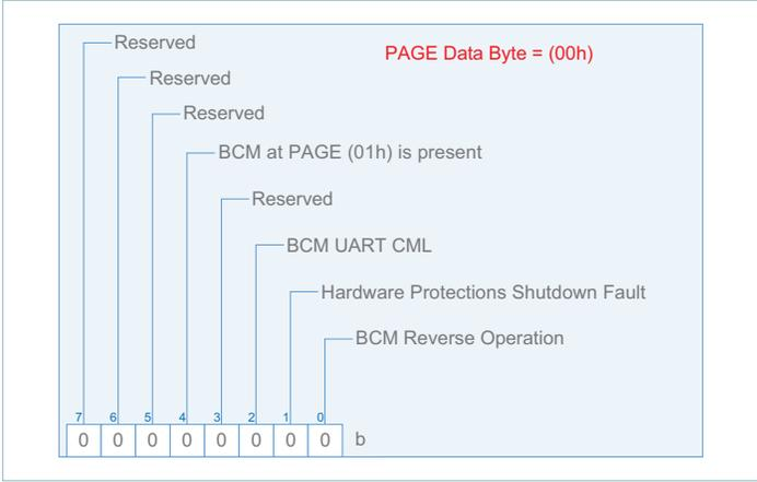
When the PAGE COMMAND (00h) data byte is equal to (00h), the BCM Reverse operation, Analog Controller Shut-Down Fault, and BCM UART CML bit will return the result of the active BCM. The BCM UART CML will also be asserted if the active BCM stops responding. The BCM must communicate at least once to the internal controller in order to trigger this FAULT. The BCM UART CML can be cleared using the PAGE (00h) CLEAR\_FAULTS (03h) Command.
