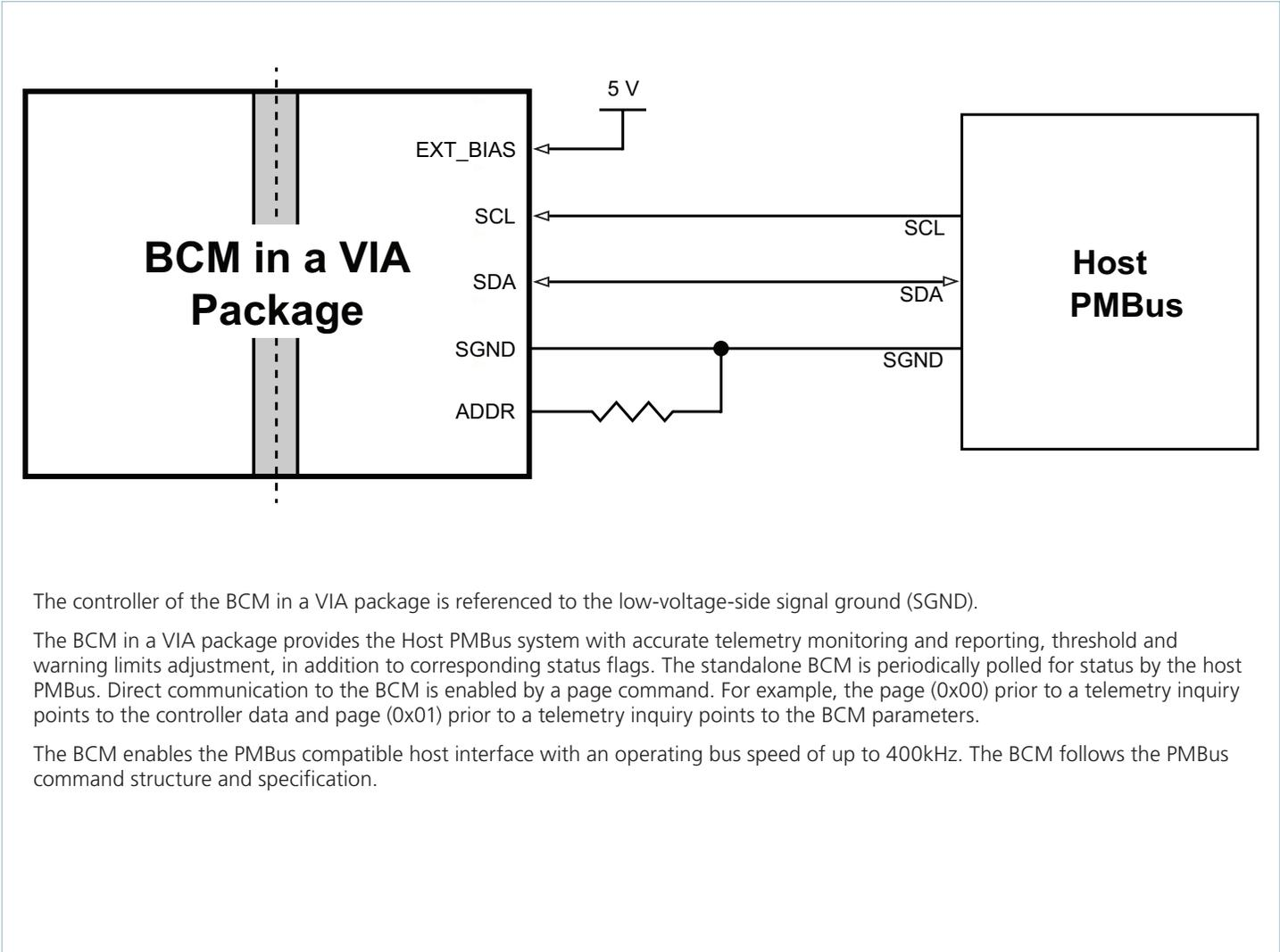
The controller of the BCM in a VIA package is referenced to the low-voltage-side signal ground (SGND).
