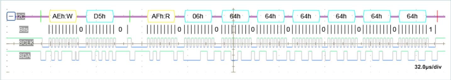
Figure 6 — SET\_ALL\_THRESHOLDS COMMAND (D5h)\_READ BLOCK PROTOCOL
