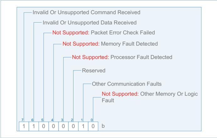
Unsupported bits are indicated above. A one indicates a fault. The STATUS\_CML data byte will be asserted when an unsupported PMBus® command or data or other communication fault occurs.
