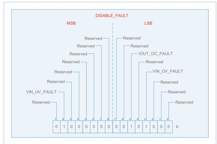
Unsupported bits are indicated above. A one indicates that the supervisory fault associated with the asserted bit is disabled.
