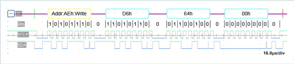
Figure 3 — TON\_DELAY COMMAND (D6h)\_WRITE WORD PROTOCOL
