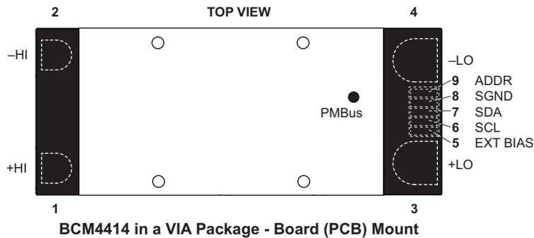
Note: The dot on the VIA housing indicates the location of the signal pin 9.
