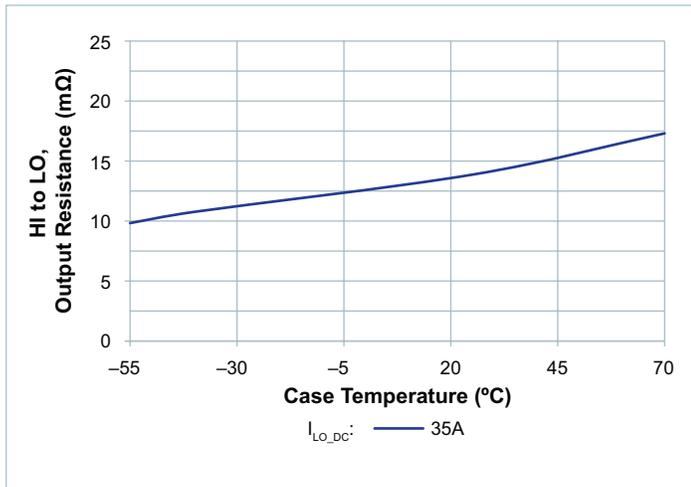
Figure 12 —  $R_{LO}$  vs. temperature; nominal  $V_{HI\_DC}$ ,  $I_{LO\_DC} = 35A$
