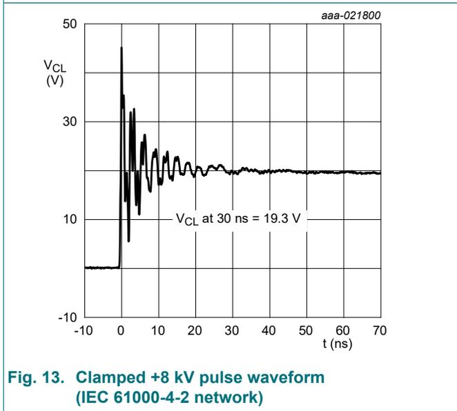
Fig. 13. Clamped +8 kV pulse waveform (IEC 61000-4-2 network)
