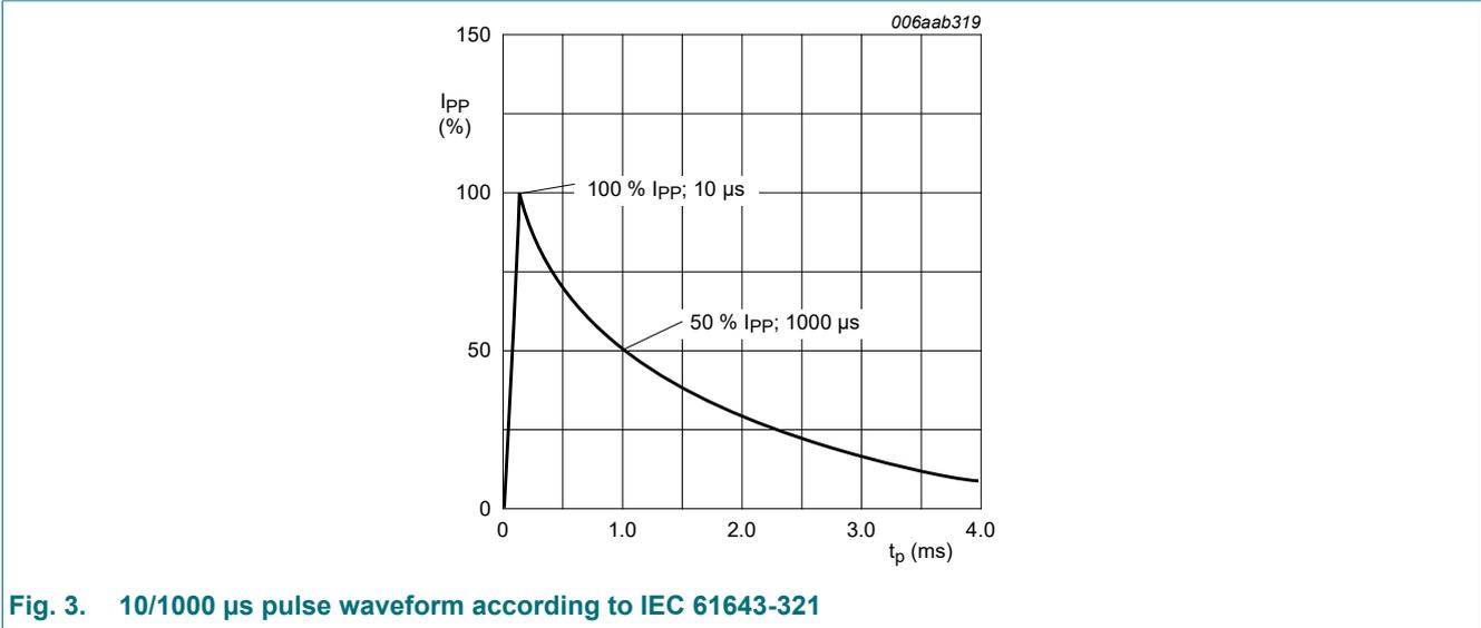
Fig. 3. 10/1000  $\mu$ s pulse waveform according to IEC 61643-321
