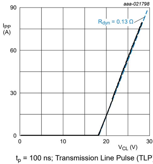
Fig. 8. Positive clamping voltage (TLP); typical values
