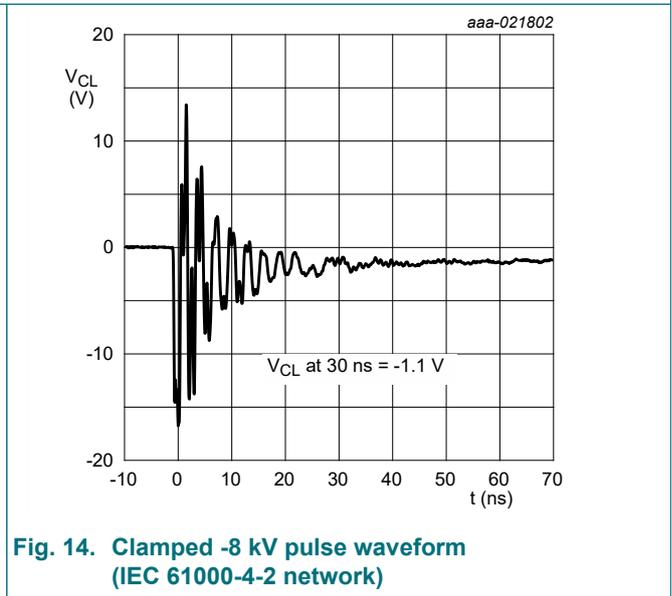
Fig. 14. Clamped -8 kV pulse waveform (IEC 61000-4-2 network)
