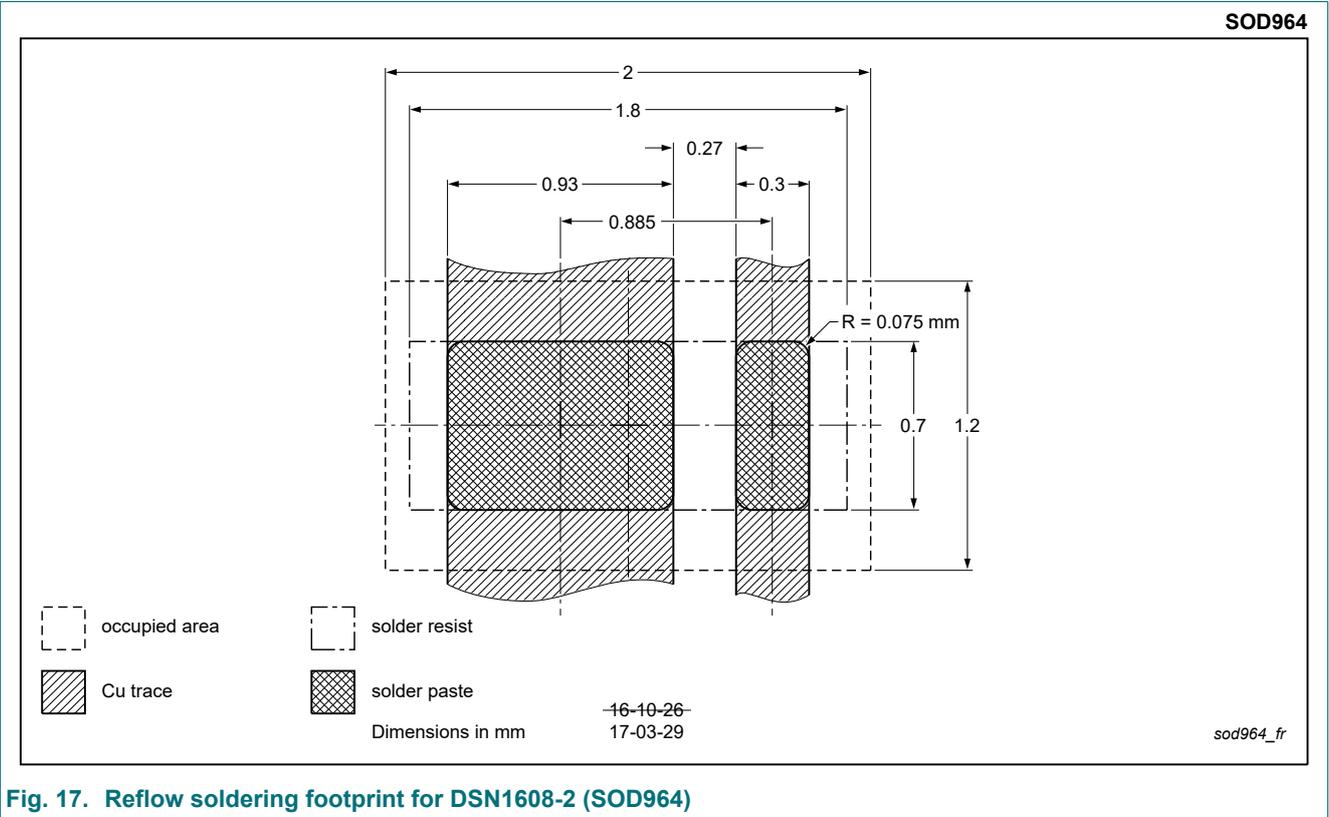
**Fig. 17. Reflow soldering footprint for DSN1608-2 (SOD964)**
