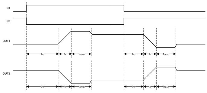
Figure 6. Propagation Delay Time
