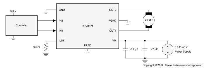
Figure 7. Typical Connections
