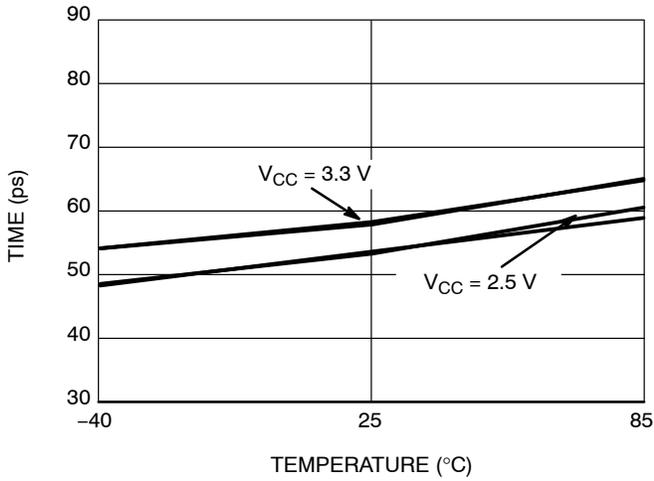
**Figure 5. Rise/Fall Time vs. Temperature and Power Supply**
