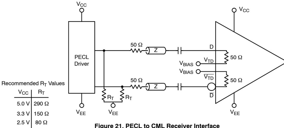
Figure 21. PECL to CML Receiver Interface
