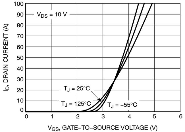
Figure 2. Transfer Characteristics
