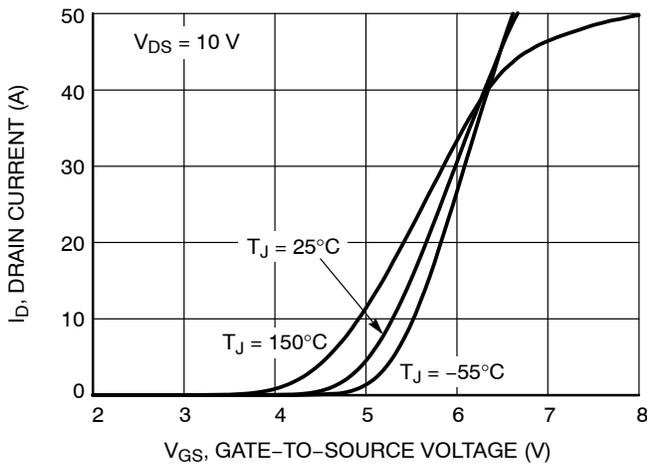
Figure 5. Transfer Characteristics
