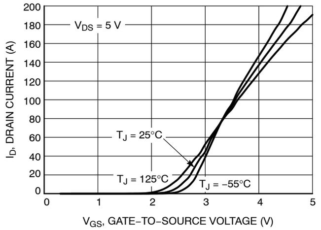
Figure 2. Transfer Characteristics
