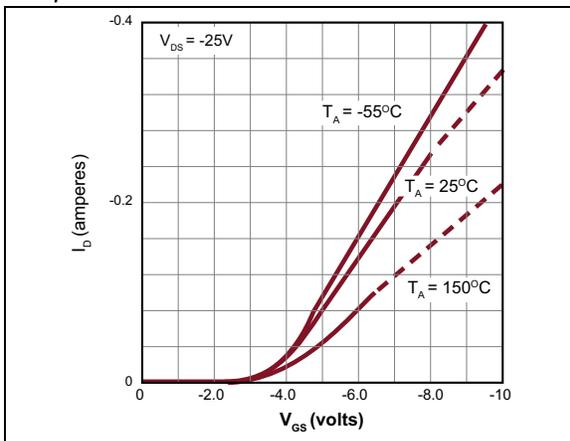
**FIGURE 2-8:** Transfer Characteristics.
