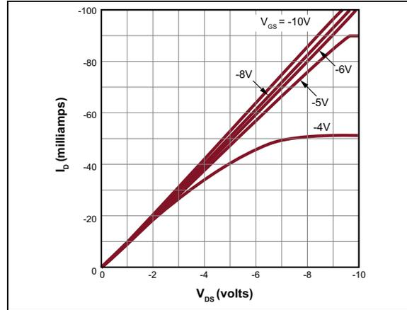
**FIGURE 2-4:** Saturation Characteristics.
