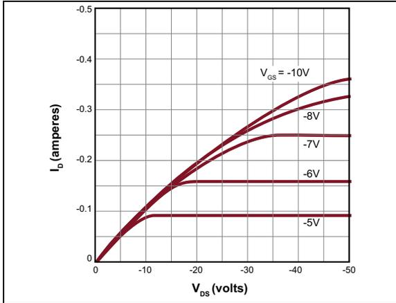
**FIGURE 2-1:** Output Characteristics.
