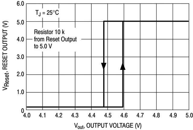
Figure 10. Reset Output versus Regulator Output Voltage
