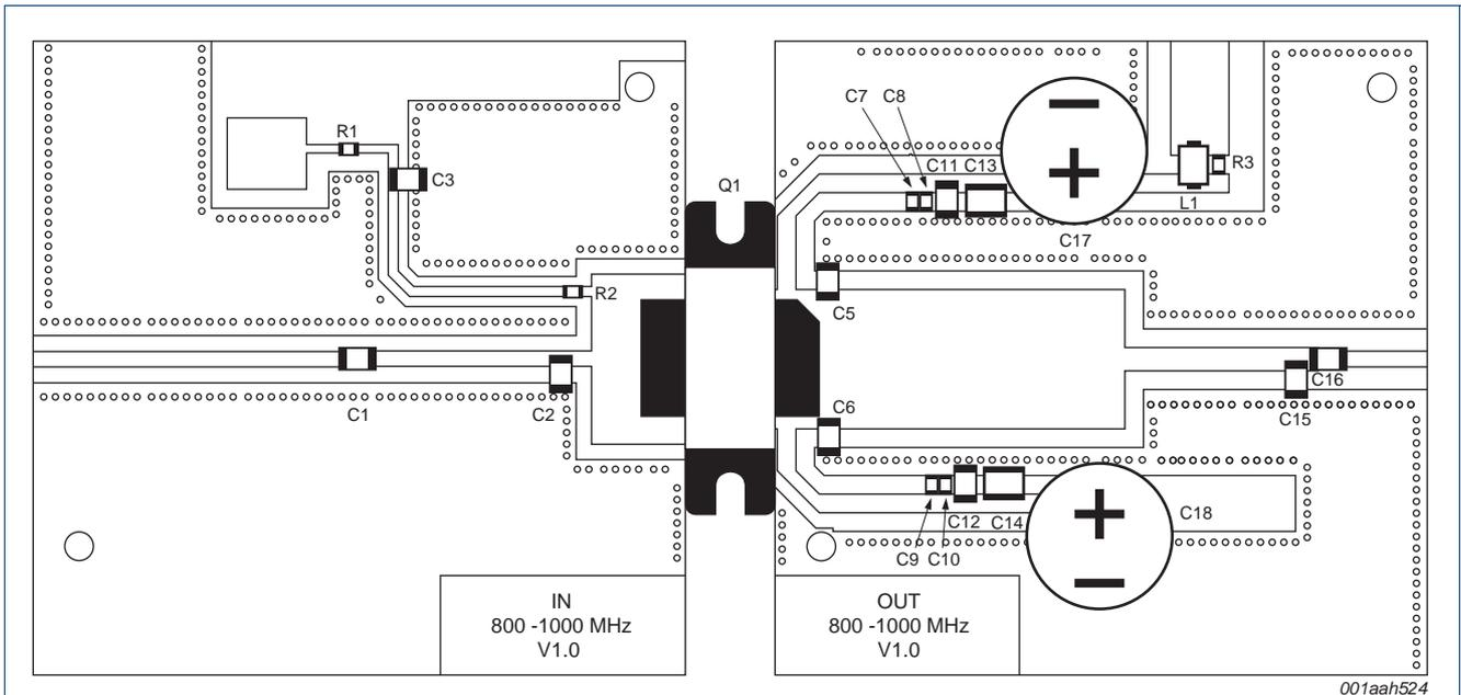
The striplines are on a double copper-clad Taconic RF35 Printed-Circuit Board (PCB) with  $\epsilon_r = 3.5$  and thickness = 0.76 mm.
