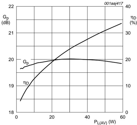
$V_{DS} = 28$  V;  $I_{Dq} = 1400$  mA;  $f = 881$  MHz ( $\pm 5$  MHz); carrier spacing 10 MHz.
