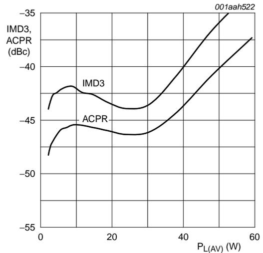
$V_{DS} = 28$  V;  $I_{Dq} = 1400$  mA;  $f = 881$  MHz ( $\pm 5$  MHz); carrier spacing 10 MHz.
