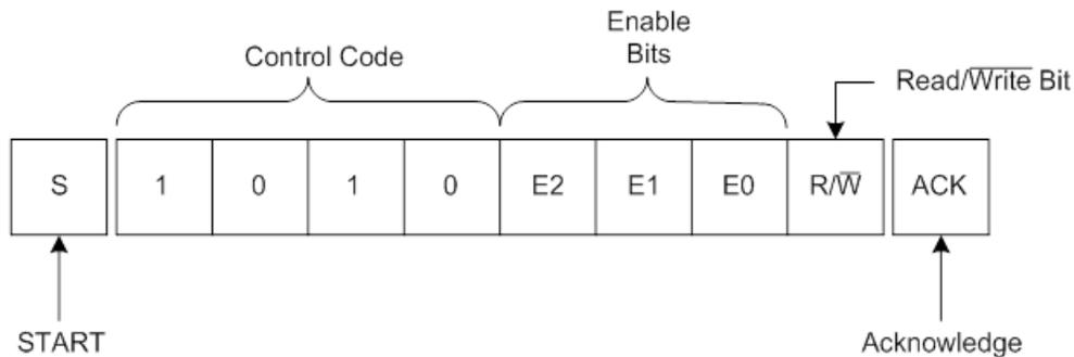
Upon receiving a "1010", the chip enable bits, and the R/W bit, the device performs an acknowledge by pulling the SDA line low during the 9th clock pulse. As stated above, the device will now be set for either a read or a write operation by the R/W bit.
