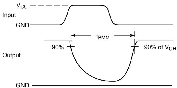
Figure 10.  $t_{BMM}$  (Time Break-Before-Make)
