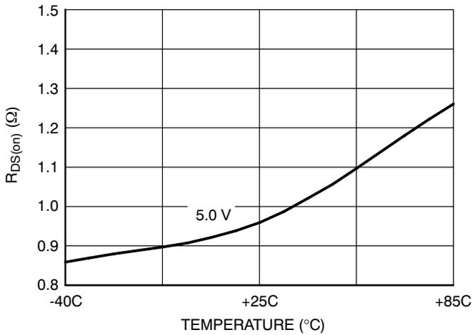
Figure 4. Delta  $R_{DS(on)}$  @  $V_{CC} = 5.0$  V
