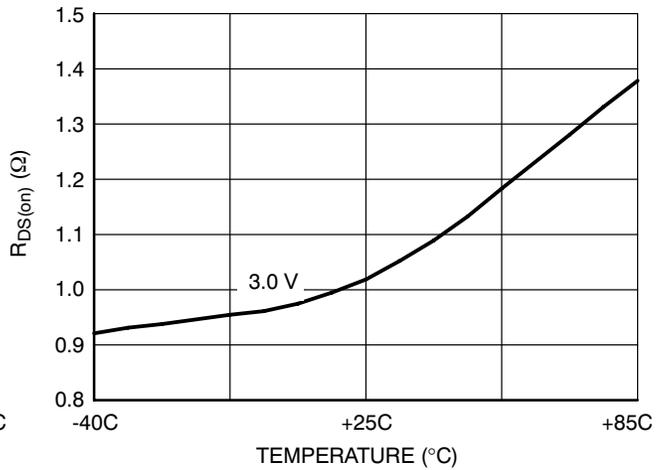
Figure 5. Delta  $R_{DS(on)}$  @  $V_{CC} = 3.0$  V
