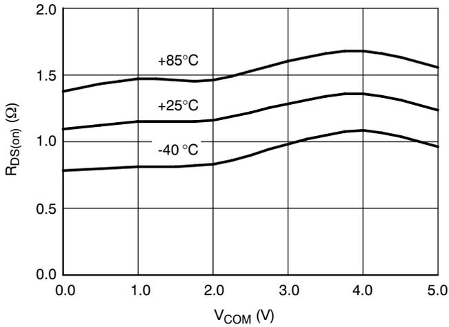
Figure 2. Low  $R_{DS(on)}$  @  $V_{CC} = 5.0$  V
