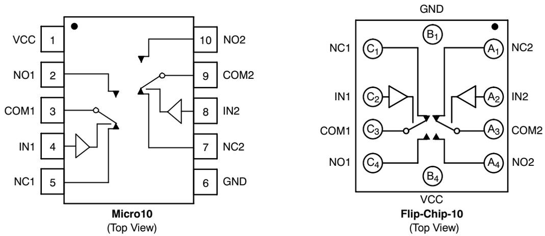
Figure 1. Device Circuit Diagrams and Pin Configurations
