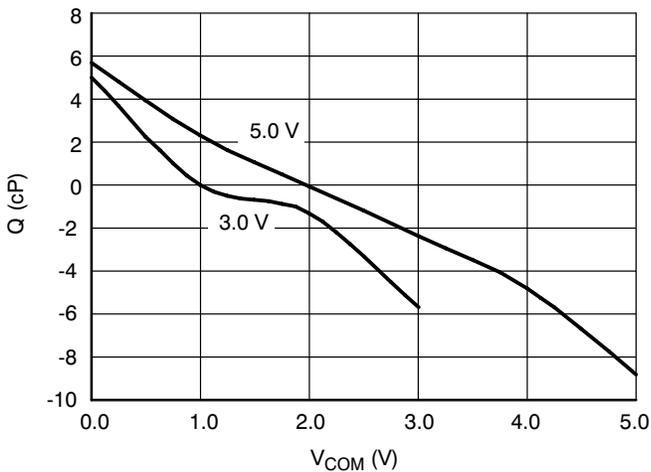
Figure 6. Charge Injection
