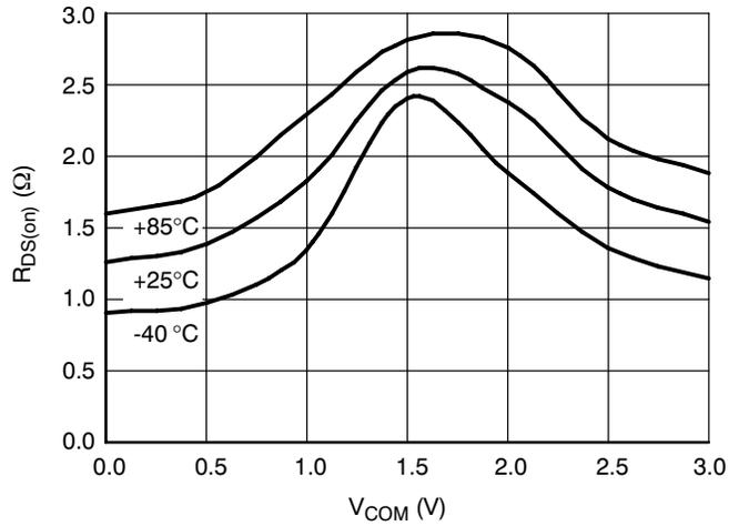
Figure 3. Low  $R_{DS(on)}$  @  $V_{CC} = 3.0$  V
