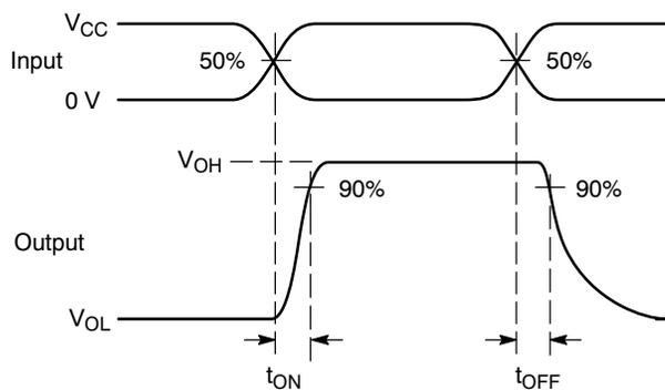
Figure 11.  $t_{ON}/t_{OFF}$
