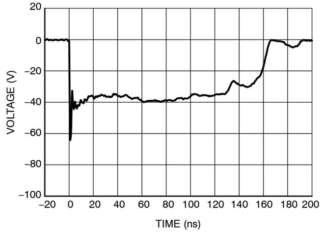
**Figure 8. IEC61000-4-2 -8 kV Contact ESD Clamping Voltage**
