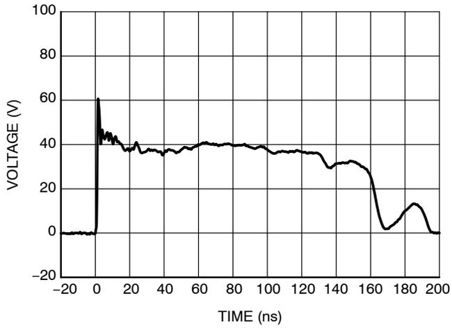
**Figure 7. IEC61000-4-2 +8 kV Contact ESD Clamping Voltage**
