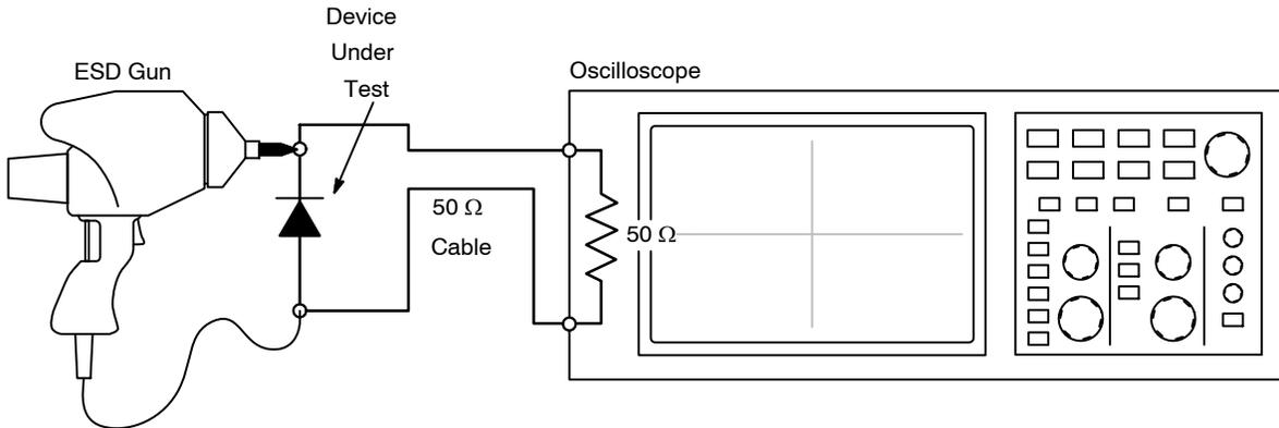
Figure 10. Diagram of ESD Clamping Voltage Test Setup
