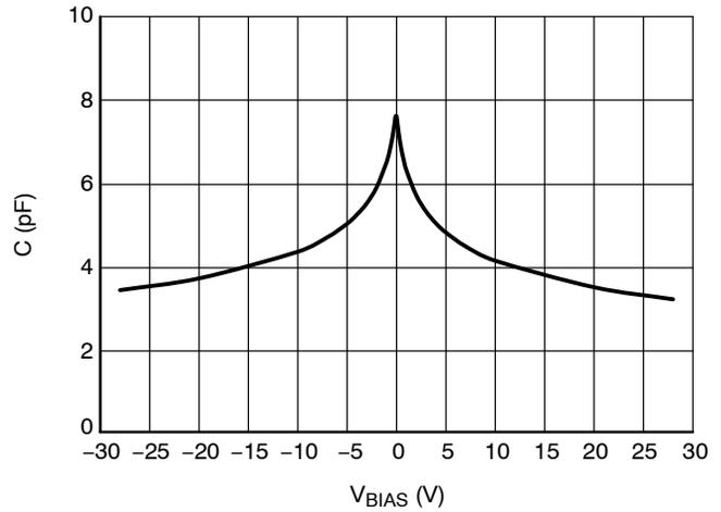
Figure 2. CV Characteristics
