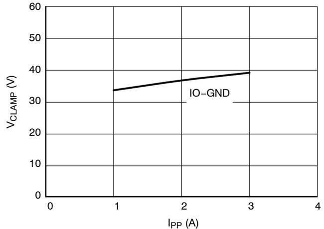
Figure 6. Clamping Voltage vs. Peak Pulse Current (8/20  $\mu\text{s}$ )
