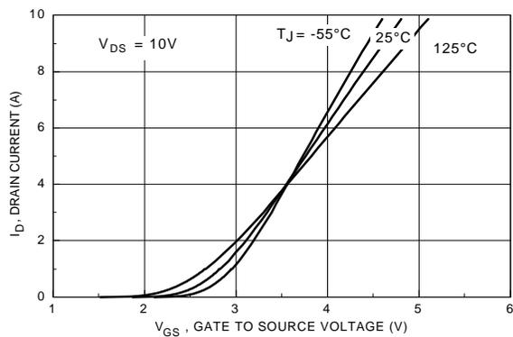
Figure 5. Transfer Characteristics
