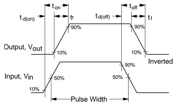
**Figure 12. Switching Waveforms**
