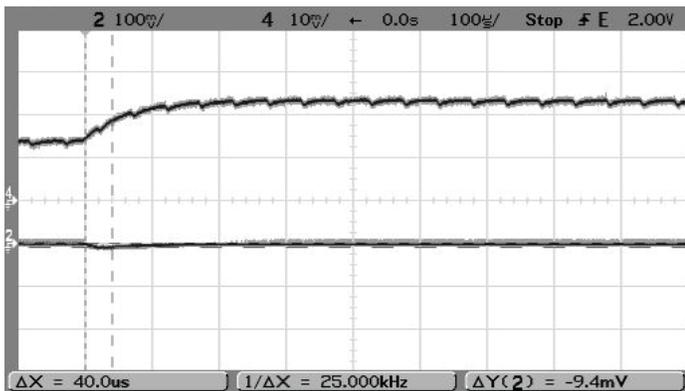
Step Load Transient Response ( $V_{in}=2.6V$ ,  $V_{out}=0.9V$ ,  $C_{load}=0$ ,  $I_{out}=1A$  to  $0.5A$ ,
