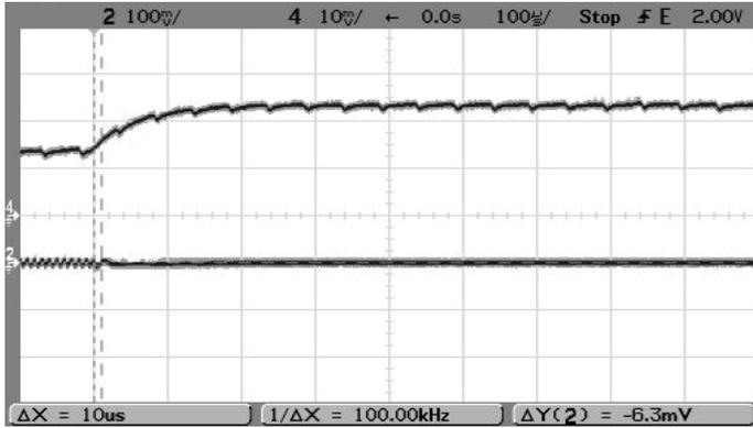
Step Load Transient Response (Vin=12V, Vout=0.9V, Cload=0, Iout=1A to 0.5A, Ta=+25°C.) Trace 2=Vout, 100 mV/div. Trace 4=Iout, 0.5A/div.
