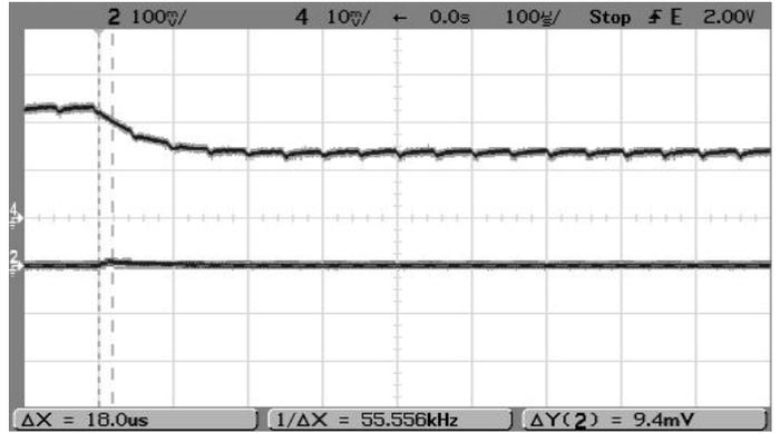
Step Load Transient Response (Vin=14V, Vout=0.9V, Cload=0, Iout=0.5A to 1A, Ta=+25°C.) Trace 2=Vout, 100 mV/div. Trace 4=Iout, 0.5A/div.
