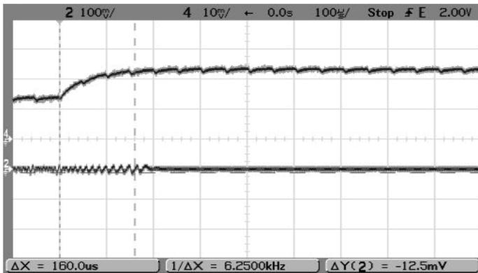
Step Load Transient Response (Vin=14V, Vout=0.9V, Cload=0, Iout=1A to 0.5A, Ta=+25°C.) Trace 2=Vout, 100 mV/div. Trace 4=Iout, 0.5A/div.
