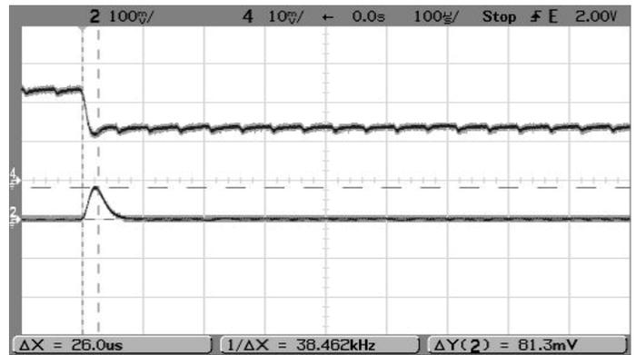
Step Load Transient Response (Vin=12V, Vout=2.5V, Cload=0, Iout=0.5A to 1A, Ta=+25°C.) Trace 2=Vout, 100 mV/div. Trace 4=Iout, 0.5A/div.
