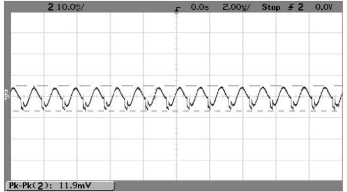
Output Ripple and Noise ( $V_{in}=14V$ ,  $V_{out}=0.9V$ ,  $I_{out}=1A$ ,  $C_{load}=0$ ,
