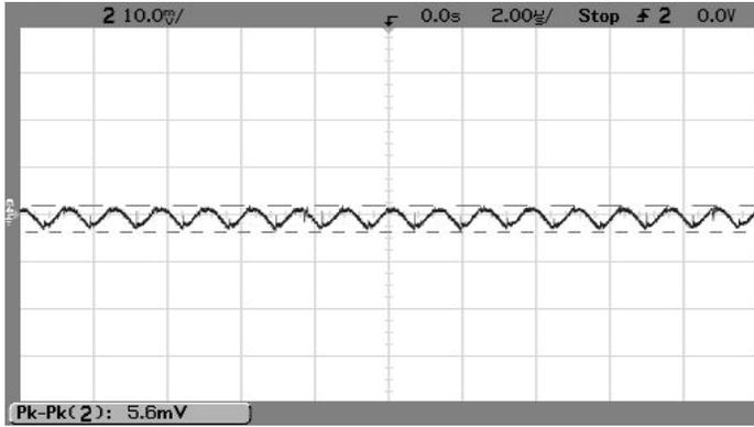
Output Ripple and Noise ( $V_{in}=12V$ ,  $V_{out}=0.9V$ ,  $I_{out}=1A$ ,  $C_{load}=0$ ,
