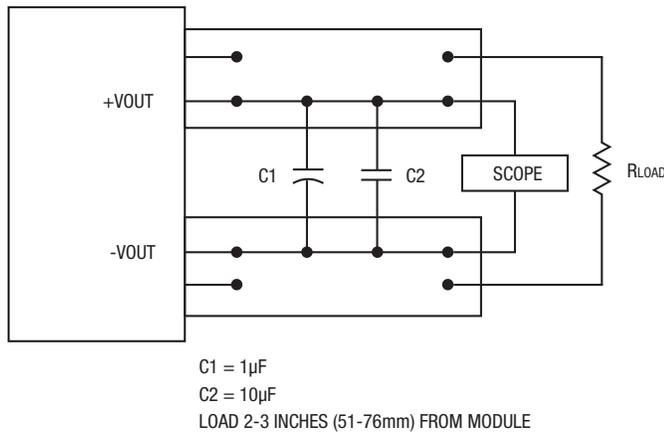
Figure 5. Measuring Output Ripple and Noise (PARD)
