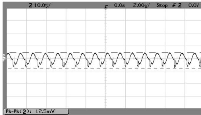
Step Load Transient Response ( $V_{in}=2.6V$ ,  $V_{out}=0.9V$ ,  $C_{load}=0$ ,  $I_{out}=0.5A$  to  $1A$ ,
