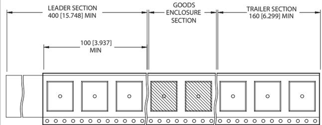
Carrier tape pockets shown are illustrative only - Refer to carrier tape diagram for actual pocket details.
