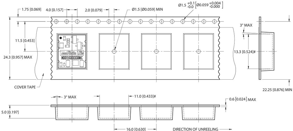
Tape & Reel specifications shall conform with current EIA-481 standard
