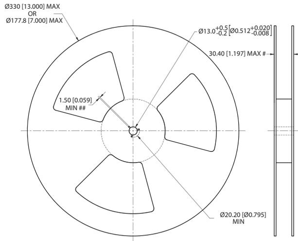
Tape & Reel specifications shall conform with current EIA-481 standard
