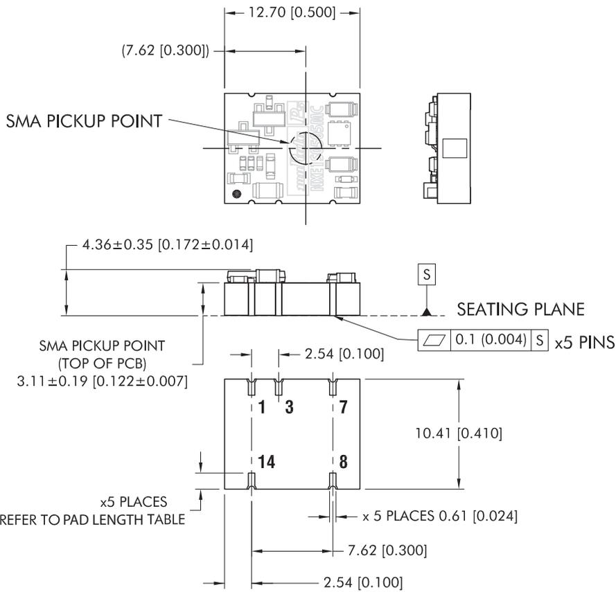
All dimensions in mm (inches), Controlling dimension is mm.
