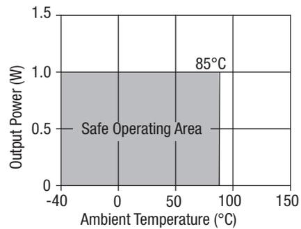
1. Derating tests carried out with a product placed on a veroboard, area 1".
