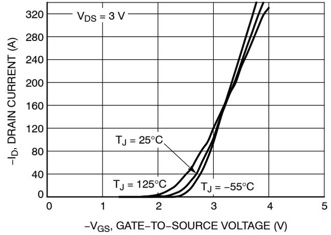
Figure 2. Transfer Characteristics
