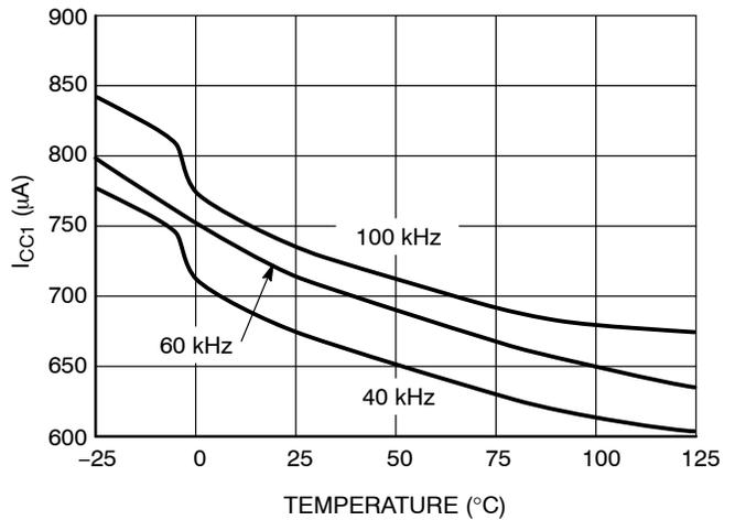
**Figure 6. I<sub>CC1</sub> vs. Temperature**
