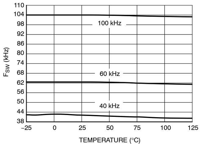
**Figure 8. Switching Frequency vs. T<sub>J</sub>**
