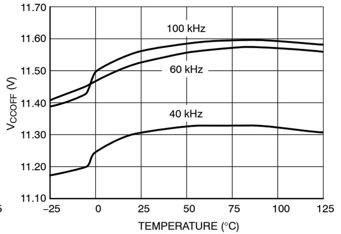
**Figure 4. V<sub>CC</sub> OFF vs. Temperature**
