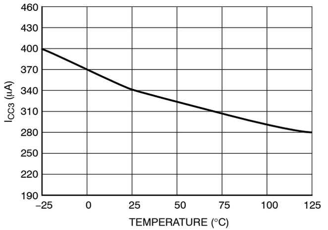
Figure 10. I<sub>CC3</sub> vs. Temperature
