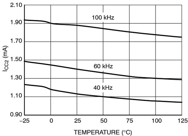
**Figure 7. I<sub>CC2</sub> vs. Temperature**
