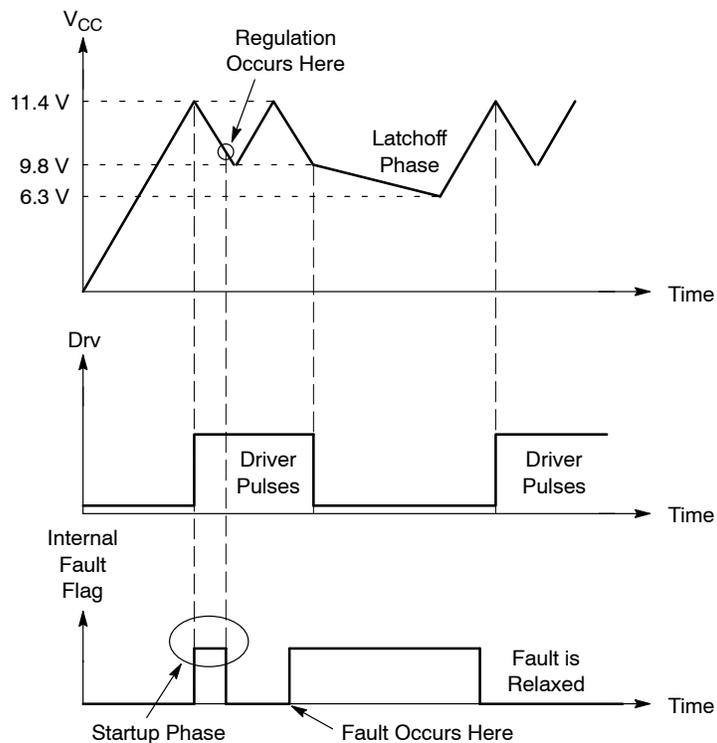
**Figure 20. If the fault is relaxed during the V<sub>CC</sub> natural fall down sequence, the IC automatically resumes. If the fault persists when V<sub>CC</sub> reached UVLO<sub>L</sub>, then the controller cuts everything off until recovery.**
