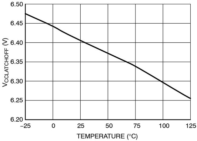
Figure 9. V<sub>CC</sub> Latchoff vs. Temperature
