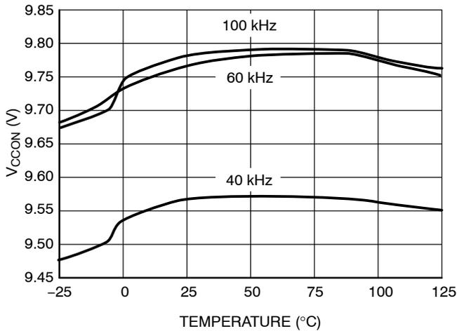
**Figure 5. V<sub>CC</sub> ON vs. Temperature**
