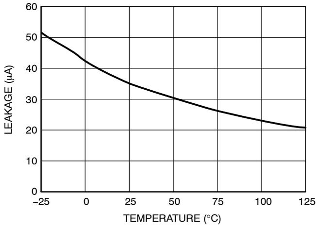
**Figure 3. HV Pin Leakage Current vs. Temperature**
