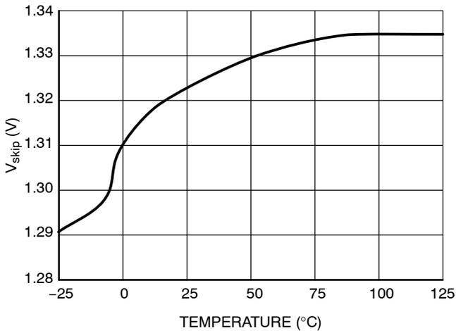
Figure 13. V<sub>skip</sub> vs. Temperature
