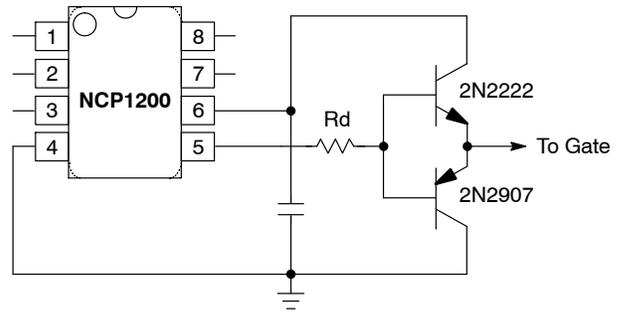
**Figure 26. Improving Both Turn-On and Turn-Off Times**
