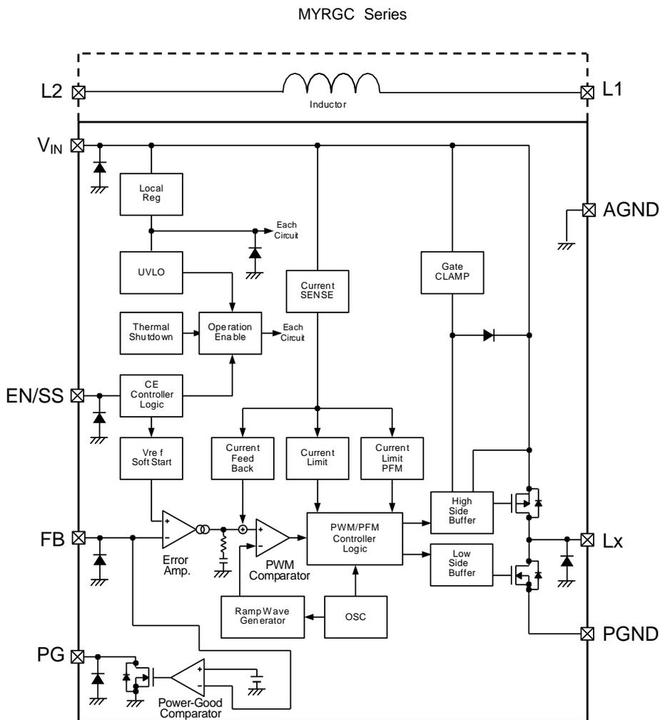
\*Diodes inside the circuit are an ESD protection diodes and a parasitic.
