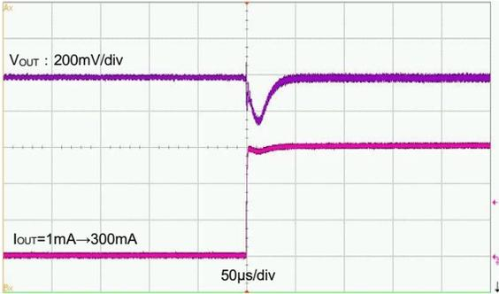
MYRGC075050P/Q ( $V_{IN}=12V$ ,  $V_{OUT}=5V$ ,  $I_{OUT}=300mA \rightarrow 1mA$ )
