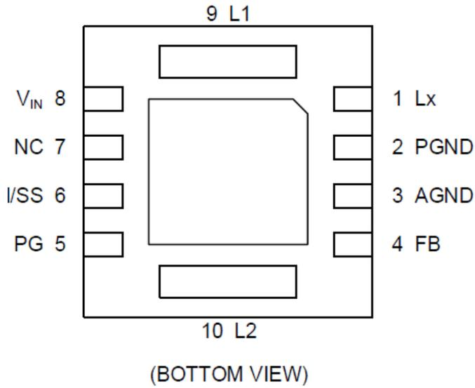
\* The dissipation pad for this package should be solder-plated in recommended mount pattern and metal masking so as to enhance mounting strength and heat release. If the pad needs to be connected to other pins, it should be connected to the GND (No. 2 and No.3) pin.
