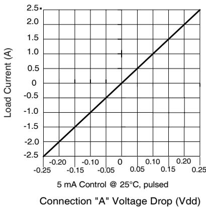
Figure 3. Linearity Characteristics
