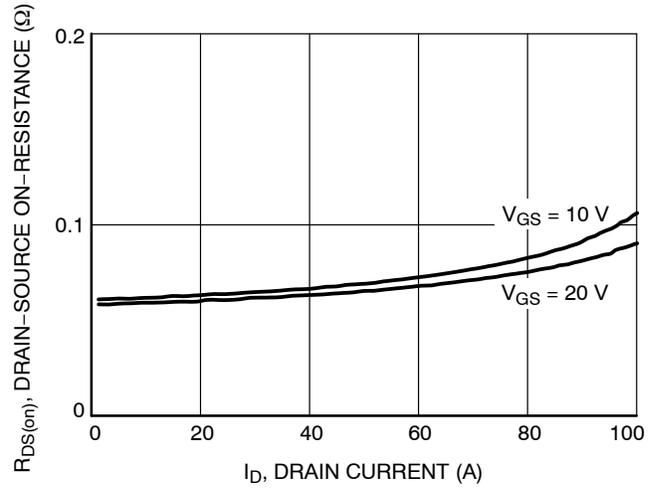
**Figure 4. On-Resistance Variation vs. Drain
