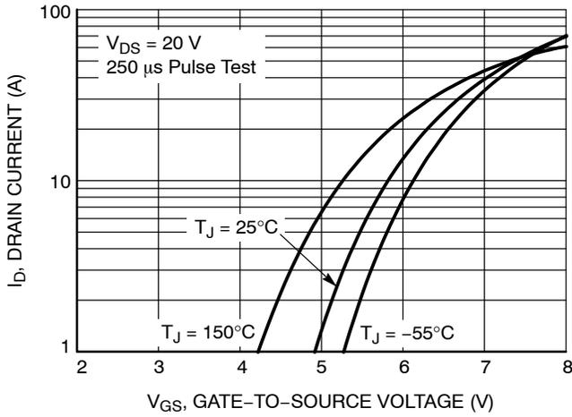
**Figure 3. Transfer Characteristics**
