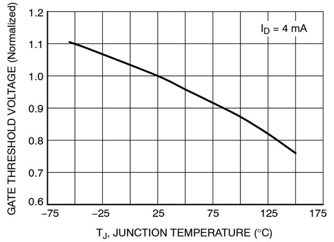
Figure 14. Normalized Gate Threshold Voltage vs. Temperature
