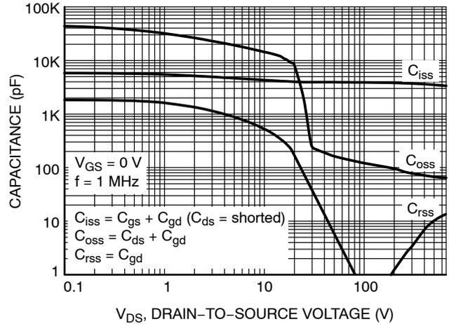
**Figure 6. Capacitance Characteristics**
