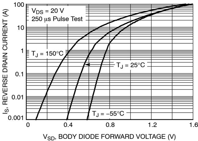
**Figure 5. Body Diode Forward Voltage
