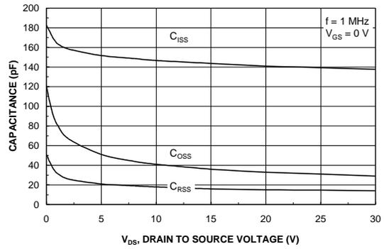
Figure 8. Capacitance Characteristics.
