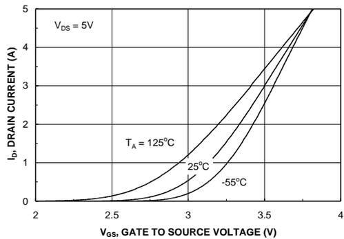
Figure 5. Transfer Characteristics.
