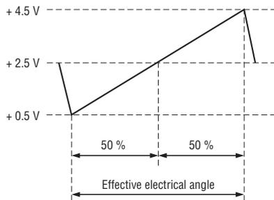
※ The output increases with CW shaft rotation.
