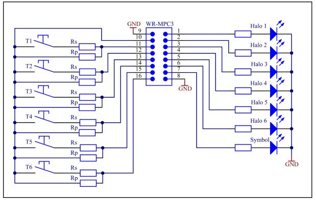
Picture 1: Internal electrical circuit of the keypad
