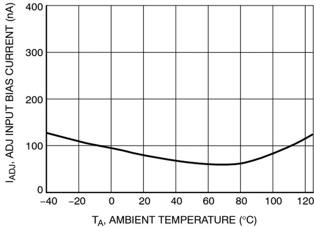
Figure 24. ADJ Input Bias Current vs. Temperature
