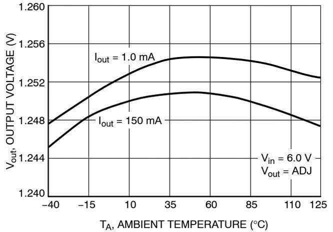
Figure 9. Output Voltage vs. Temperature ( $V_{in} = 6.0 V$ )
