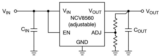
**Figure 6. Typical Application Circuit for Adjustable  $V_{out}$**
