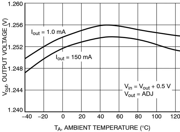
Figure 8. Output Voltage vs. Temperature ( $V_{in} = V_{out} + 0.5 V$ )
