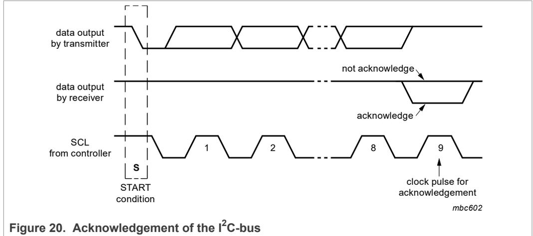
Figure 20. Acknowledgement of the I<sup>2</sup>C-bus
