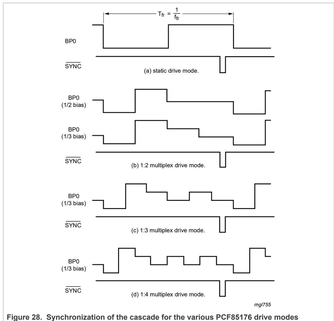
Figure 28. Synchronization of the cascade for the various PCF85176 drive modes
