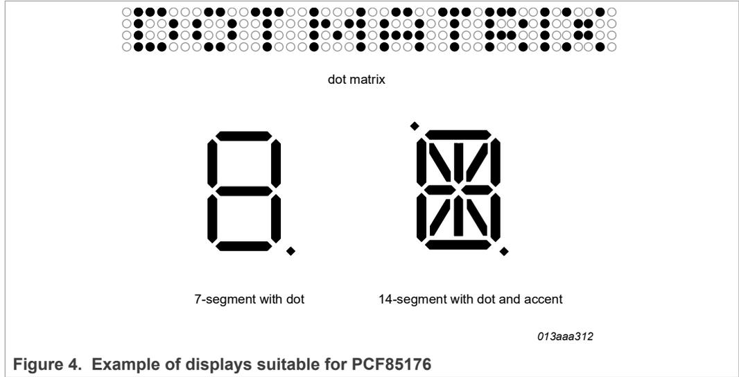
Figure 4. Example of displays suitable for PCF85176
