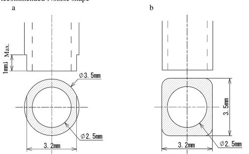
\*Nozzle with chamfering is recommended
