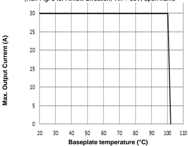
**Figure 9.** Current Derating Curve for Baseplate
