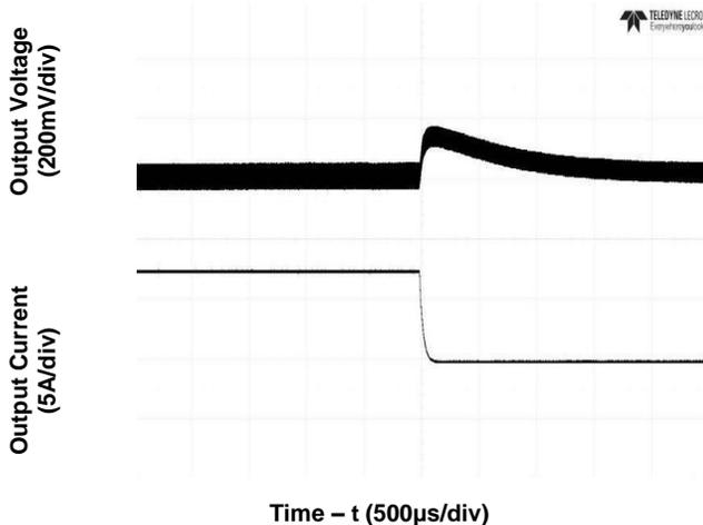
Figure 5. Transient Load Response (typical Vin, load current steps from 50% to 25% at a slew rate 0.1A/µs)
