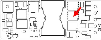
Figure 15. Temperature Monitoring Locations
