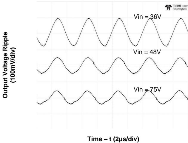
Figure 3. Output Ripple Voltage at Full Load
