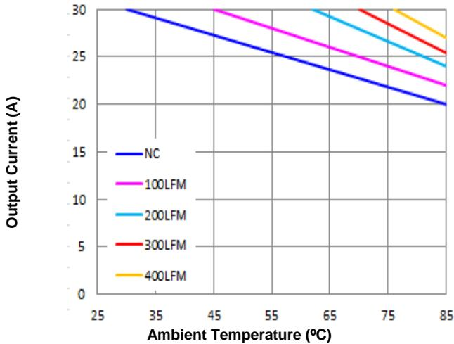
**Figure 7.** Current Derating Curve for Airflow Direction 3
