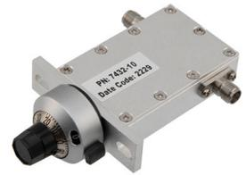
0 to 10 dB Variable Attenuator, SMA Female to SMA Female Rated to 5 Watts from 4 GHz to 8 GHz
