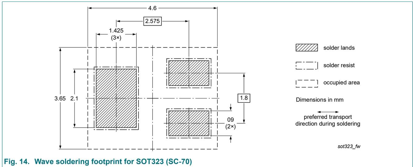
Fig. 14. Wave soldering footprint for SOT323 (SC-70)
