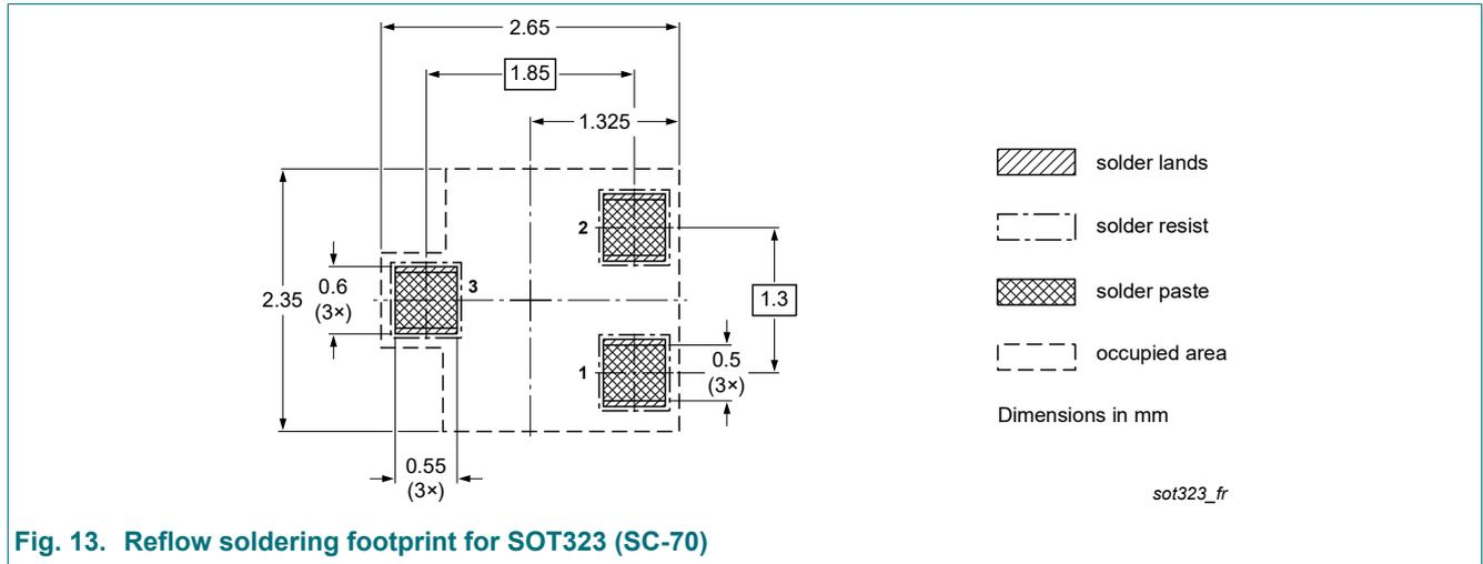
Fig. 13. Reflow soldering footprint for SOT323 (SC-70)
