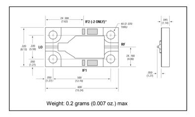
\*For base model, only IF1 port is connected. For the "-2" model, only the IF2 port is connected.
