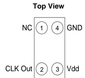
**Figure 1. Pin Assignment**
