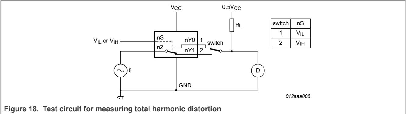
Figure 18. Test circuit for measuring total harmonic distortion
