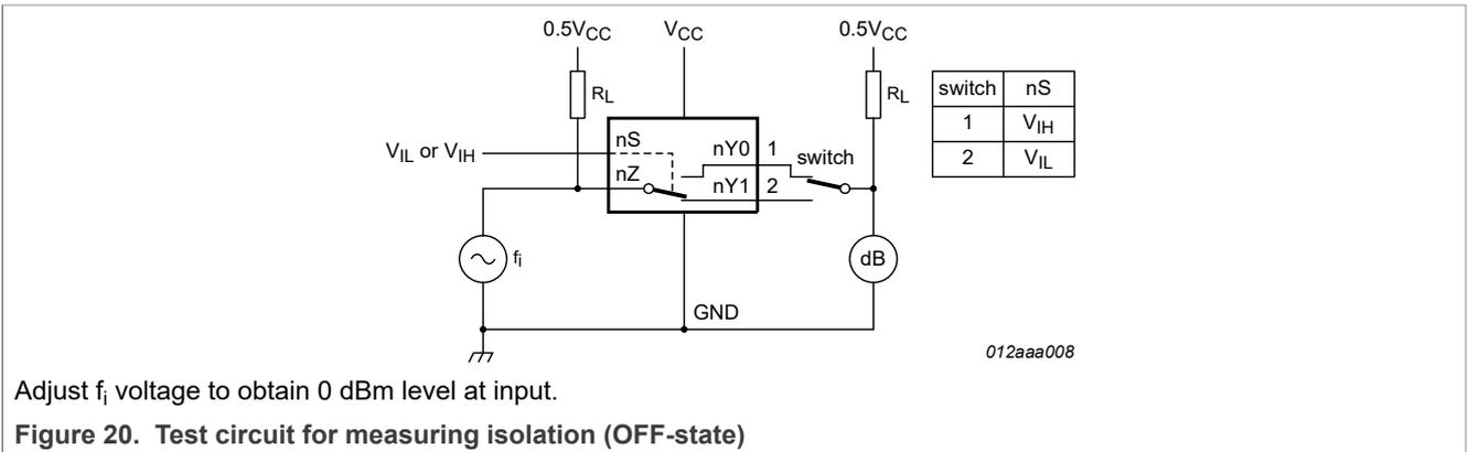
Figure 20. Test circuit for measuring isolation (OFF-state)
