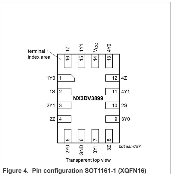
Figure 4. Pin configuration SOT1161-1 (XQFN16)
