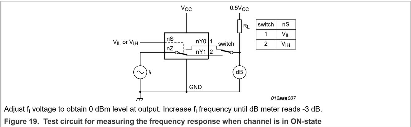
Figure 19. Test circuit for measuring the frequency response when channel is in ON-state
