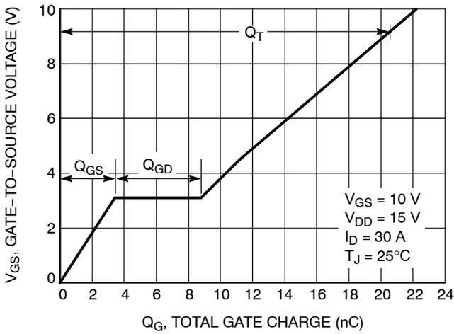
**Figure 7. Gate-to-Source and Drain-to-Source Voltage vs. Total Charge**
