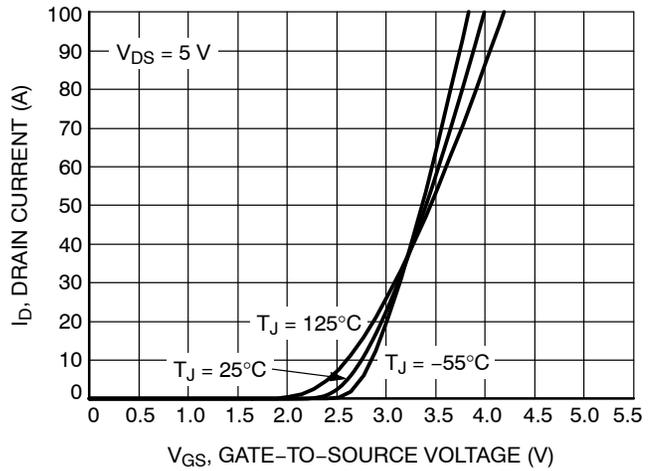
Figure 2. Transfer Characteristics
