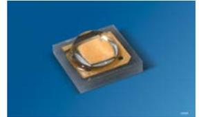
Small size high flux LED for slim designs (between 100 mA and 800 mA constant current). 94 lm (typ.), 84 lm/W (typ.) at 350 mA (4000 K).
