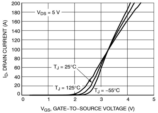
Figure 2. Transfer Characteristics
