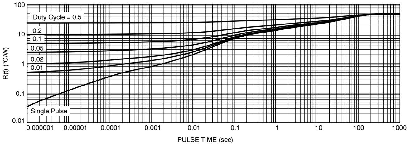
Figure 13. Thermal Characteristics
