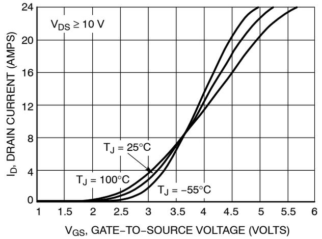
Figure 2. Transfer Characteristics
