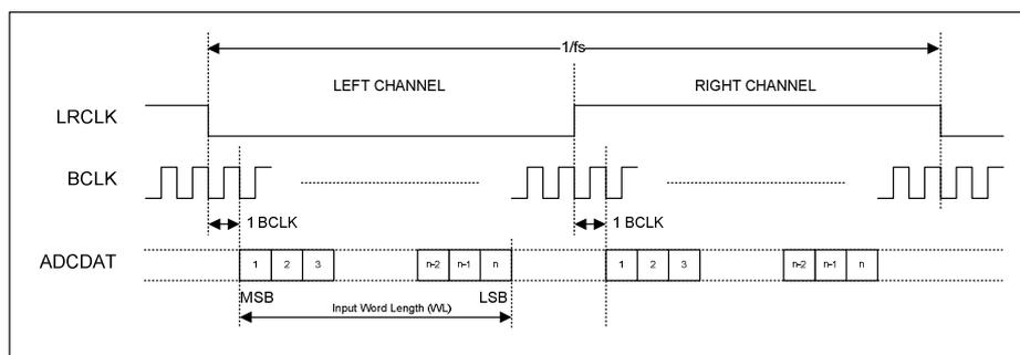
**Figure 5 I<sup>2</sup>S Digital Audio Interface format (assuming n-bit word length)**
