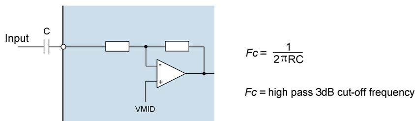
**Figure 9 Audio Input Path DC Blocking Capacitor**
