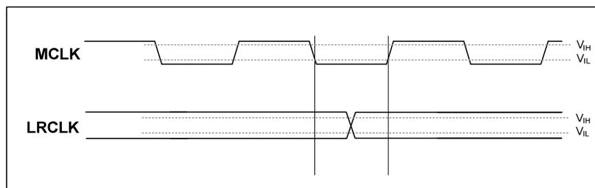
**Figure 4 Recommended LRCLK Transition Area for Optimum Performance**
