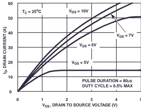
Figure 8. Saturation Characteristics
