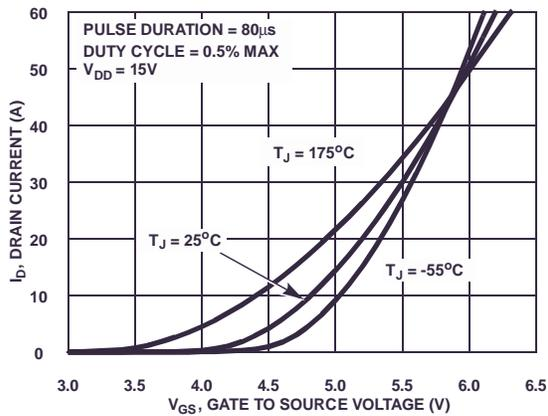
Figure 7. Transfer Characteristics
