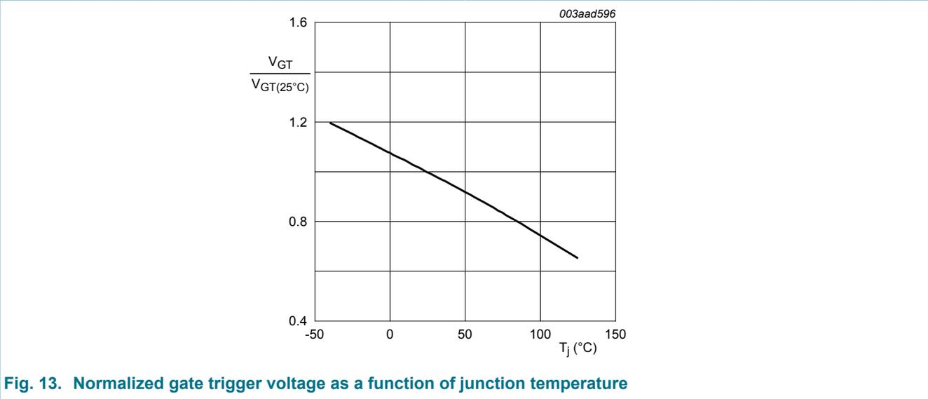
Fig. 13. Normalized gate trigger voltage as a function of junction temperature
