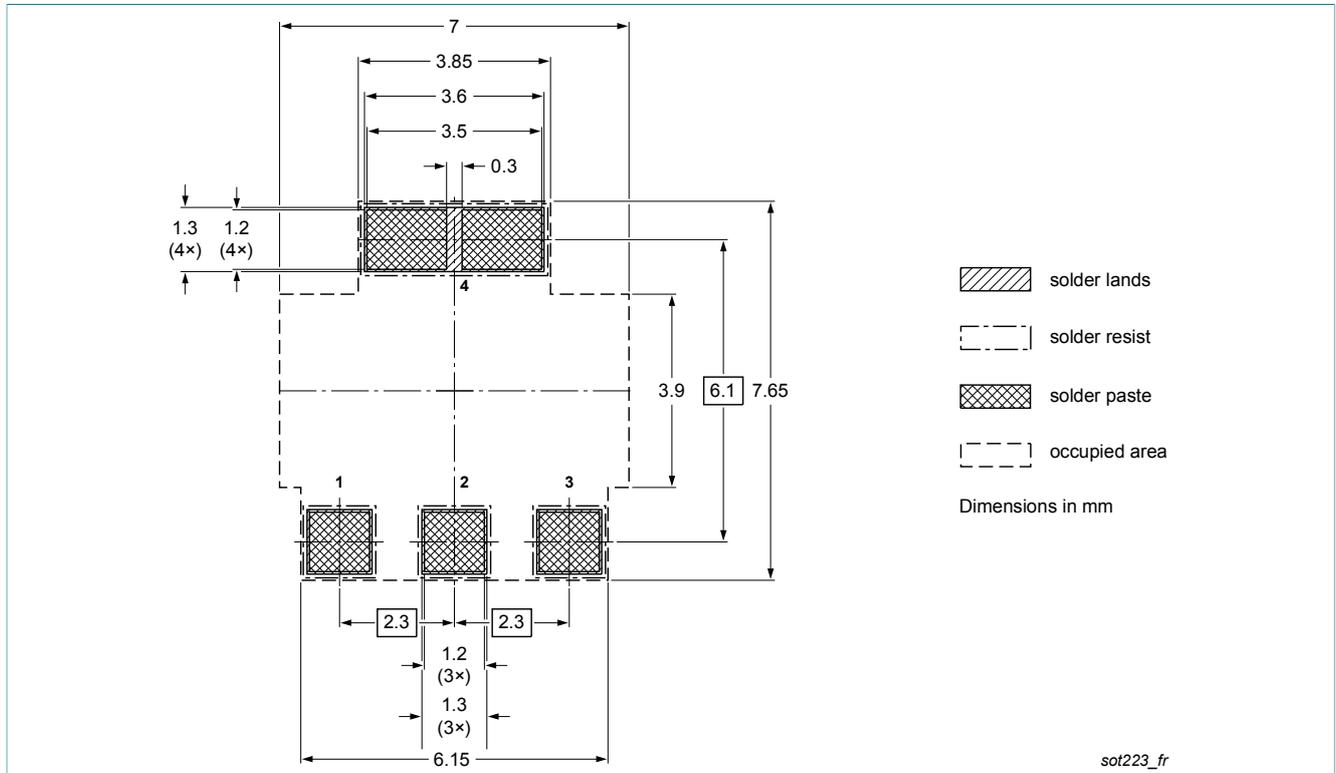
Fig. 15. Reflow soldering footprint for SC-73 (SOT223)
