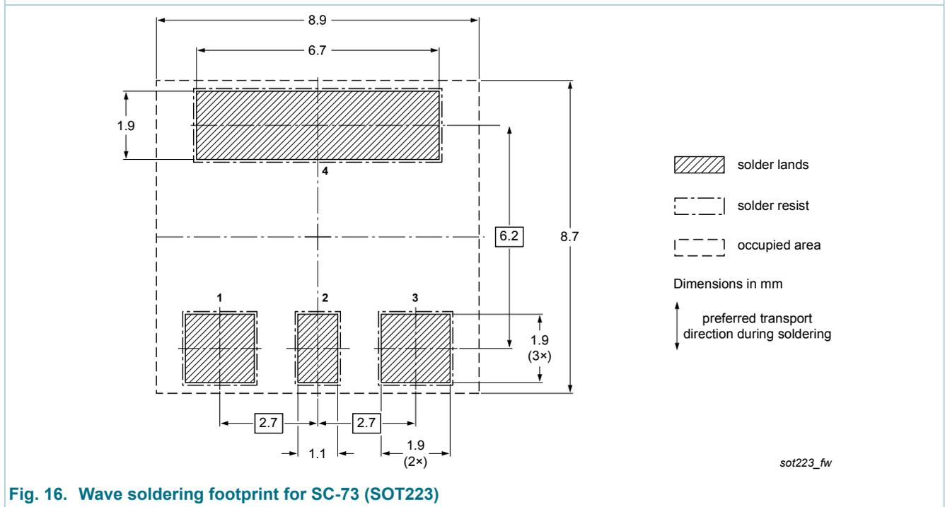
Fig. 16. Wave soldering footprint for SC-73 (SOT223)
