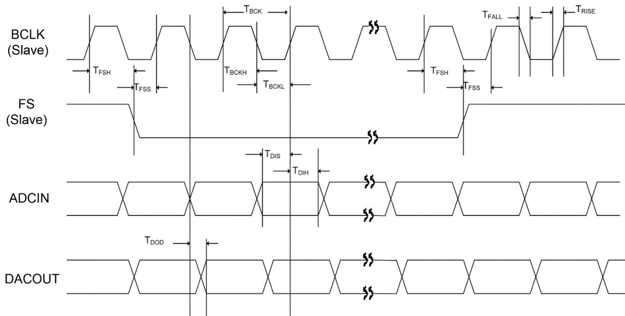
Figure 21: Digital Audio Interface Slave Mode Timing
