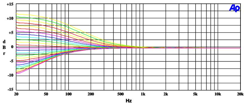
Figure 45: EQ Band 1 Gains for Lowest Cut-Off Frequency
