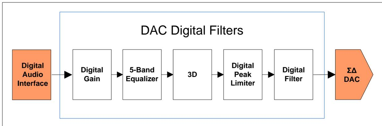
The DAC digital block uses 24-bit signal processing to generate analog audio with a 16-bit digital sample stream input. This block consists of a sigma-delta modulator, digital decimator/filter, and optional 5-band graphic equalizer/3D effects block, and a dynamic range compressor/limiter. The DAC coding scheme is in twos complement format and the full-scale output level is proportional to VDDA. With a 3.3V supply voltage, the full-scale output level is 1.0V<sub>RMS</sub>.
