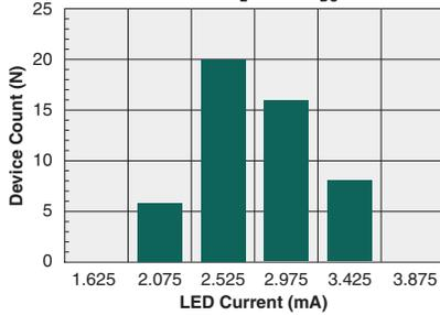
**Typical  $I_F$  for Switch Dropout**
