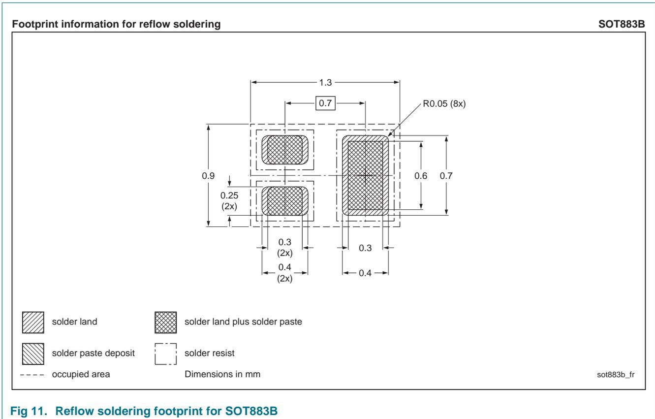
Fig 11. Reflow soldering footprint for SOT883B
