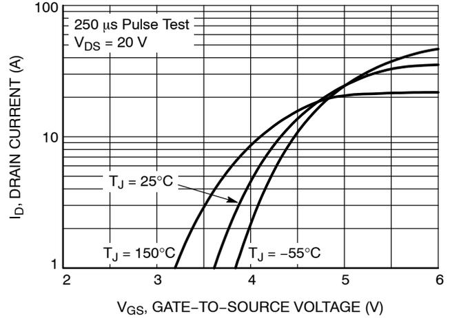
Figure 2. Transfer Characteristics
