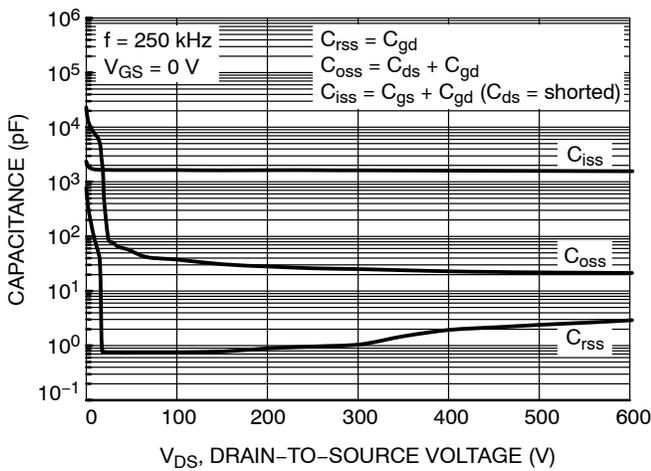
Figure 5. Capacitance Characteristics
