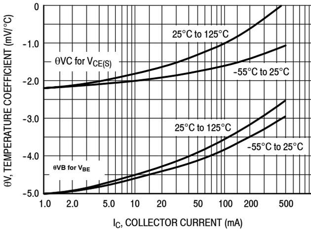
Figure 3. Temperature Coefficients
