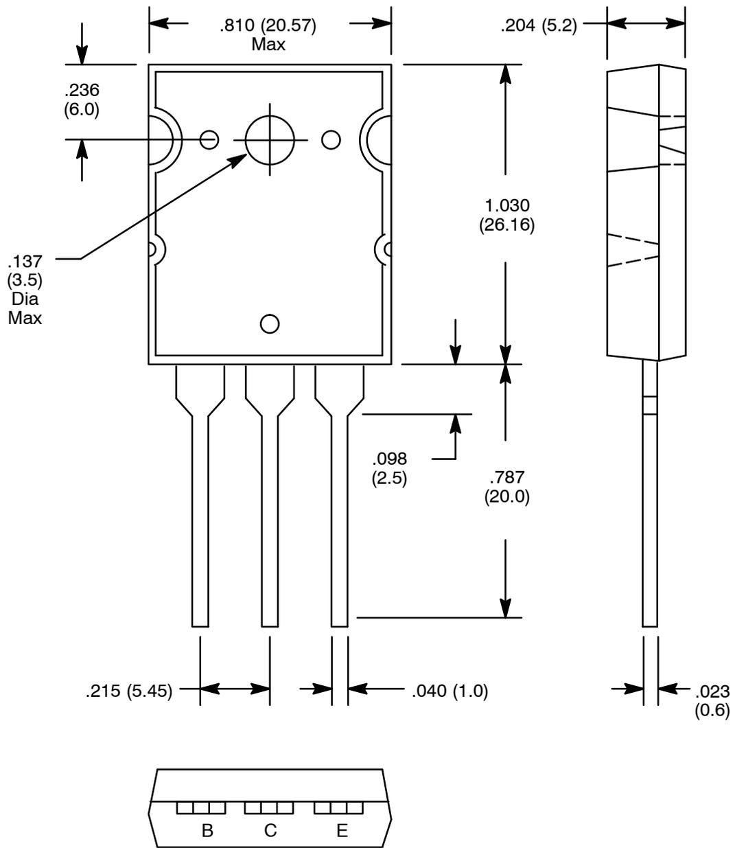
**NOTE:** Pin2 connected to heatsink
