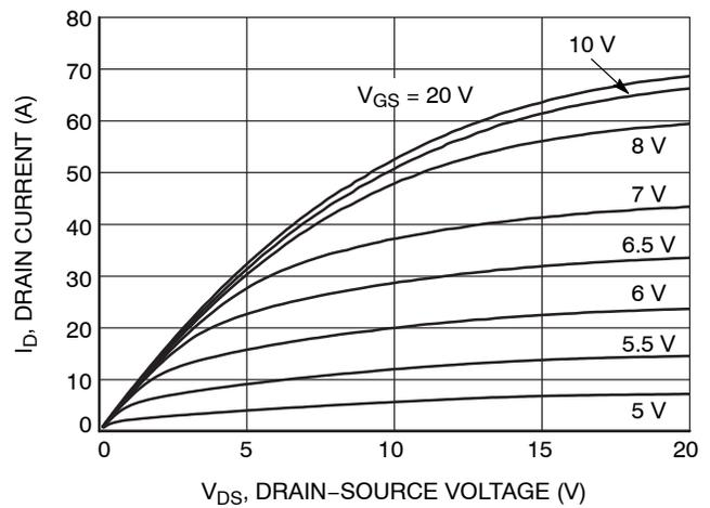
Figure 9. Saturation ( $150^{\circ}\text{C}$ )
