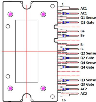
Figure 1. Pin Configuration
