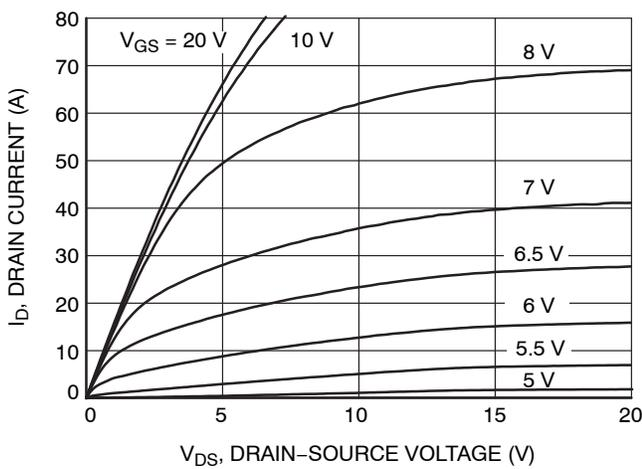
Figure 8. Saturation ( $25^{\circ}\text{C}$ )
