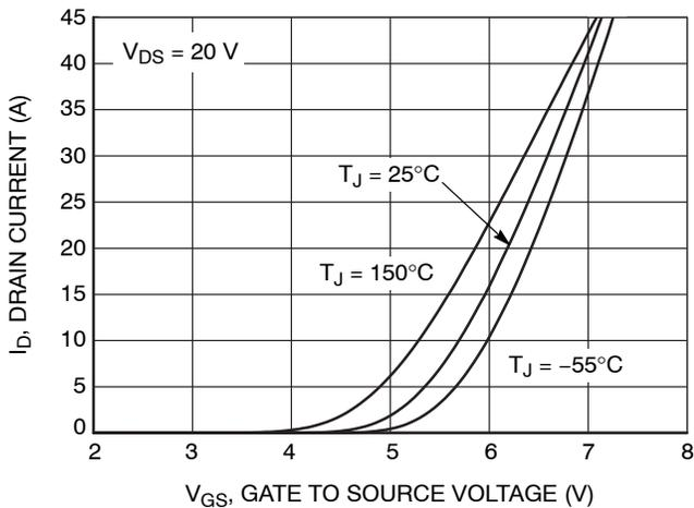
Figure 6. Transfer Characteristics
