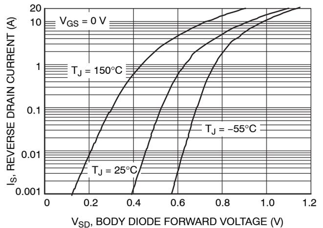
Figure 7. Forward Diode
