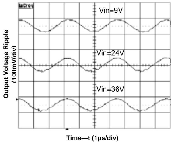
Figure 6. Output Ripple Voltage at 5V, 9A Output
