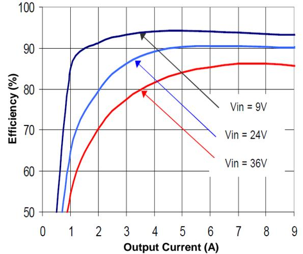
Figure 1(b). Efficiency vs. Load Current (25°C, 5V)
