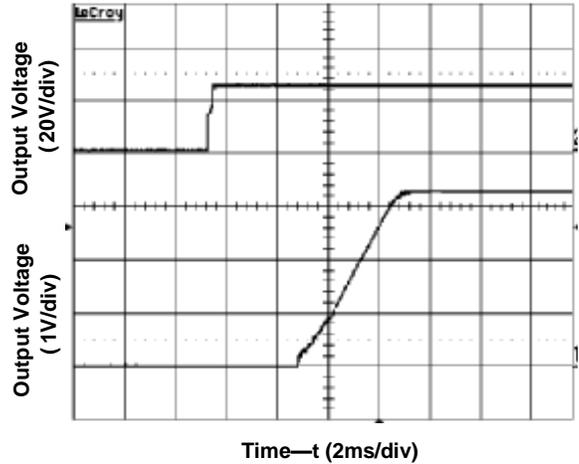
Figure 5. Start-Up from Application of Input Voltage
