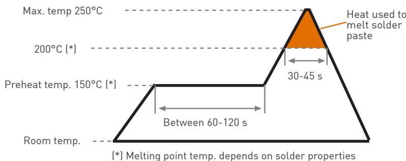
The recommended reflow profile is provided as a guideline. Optimal profile may differ due to oven type, assembly layout or other design or process variables. Customers should verify actual device performance in their specific application and reflow process. Please contact Piher if you require additional support.
