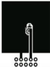
a.  $78^\circ\text{C}/\text{W}$  when mounted on a  $1\text{ in}^2$  pad of 2 oz copper on FR-4 board.
